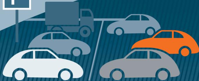
**Parking in special areas** allows for parking the car in a spot which is perpendicular to the street and would otherwise be too narrow for a driver to exit the car after being parked. The function targets the more efficient use of space in parking garages. Since the driver can exit the car in front of the parking spot, the function allows cars to be parked closer together.
